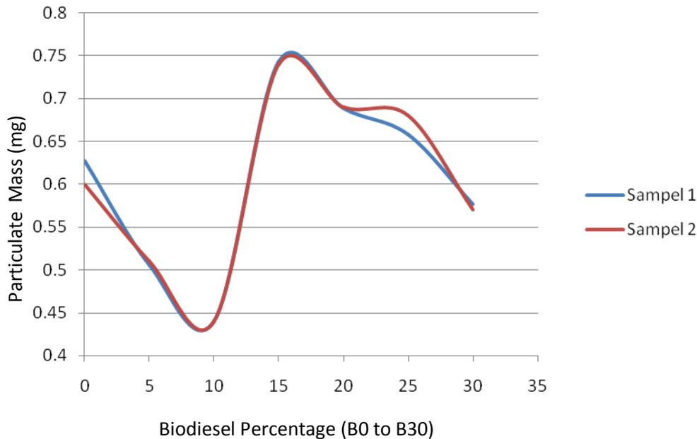
Figure 2. Graphic of Particulate Mass vs Biodiesel Percentage
