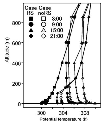
Fig. 7. Vertical profiles of potential temperature at Nerima (see Fig. 6).
