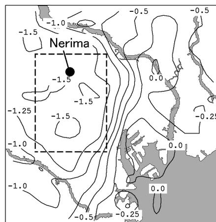
Fig. 6. Temperature difference (Case RS - Case VCR0) at 15:00 LST at 4.5 m above ground level.
