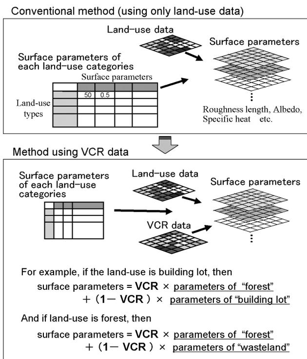
Fig. 3. Schematic diagram of the parameterization of the ground surface in meteorological model by using VCR data.
