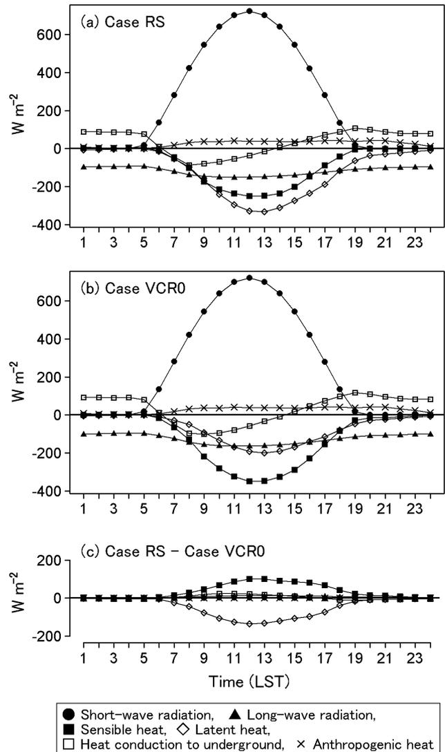
Fig. 8. Diurnal variation of surface heat budgets of (a) Case RS, (b) Case VCR0 and (c) the difference between Case RS and Case VCR0 (in the dashed-square area shown in Fig. 6).
